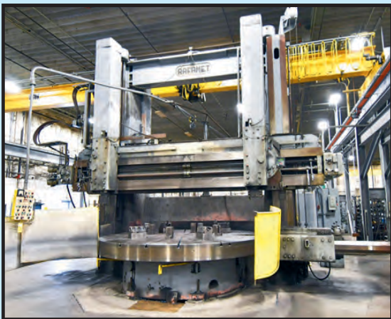
144" RAFAMET VERTICAL TURRET LATHE
